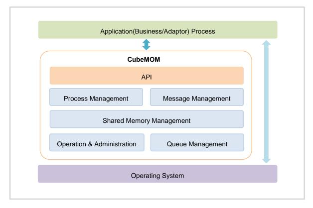
CubeMOM is message-oriented middleware for interconnection between internal and external systems. As a multi-threaded asynchronous method, it ensures high-performance and reliable message delivery. It also provides the environment for large-scale distributed application development and effective operation.
