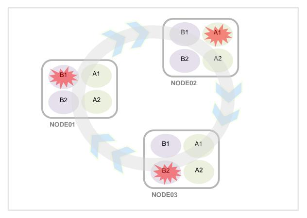
CubeMOM can configure multiple process groups on multiple nodes to increase the availability of critical tasks. By configuring multiplexing, in case of any node failure (process, queue, communication, ...), messages can be processed on the backup node without loss.
