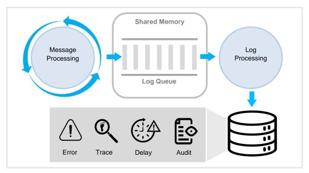
In CubeMOM, message processing and log processes are separated. The message processing process stores the logs in the queue of shared memory, and the log processing process writes the logs from the queue to disk. The message processing process has no disk input or output, which improves performance and isolates it from disk failures.
