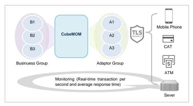
CubeMOM provides adapters for communication between internal and external systems. Adapters support various protocols (TCP, HTTP, ...) through protocol abstraction. Many functions for communication (Transport Layer Security, minimum/maximum connection, persistent/non-persistent, ...) are built-in for communication from small terminals to large servers.
